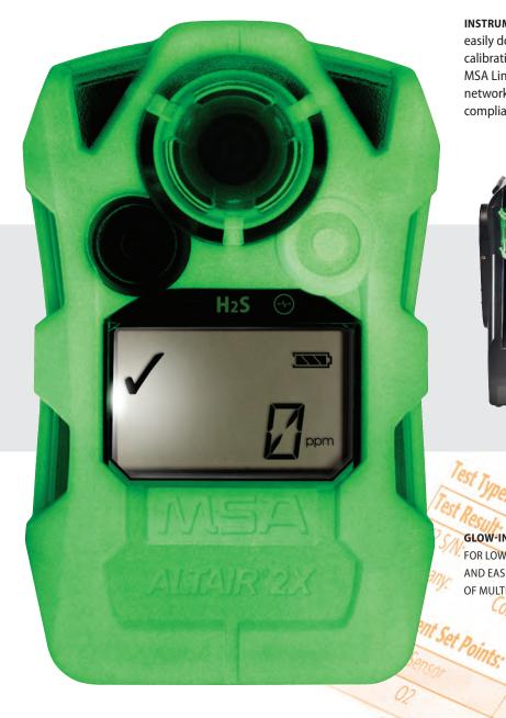
**INSTRUMENT RECORDS ARE STORED** and can be easily downloaded during periodic gas calibrations using the Galaxy GX2 test stand. MSA Link Pro Software provides full networking, traceability, proactive safety, compliance, and reporting.
